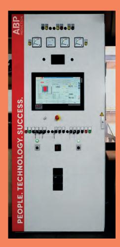
casting furnace OCC 50.2 with a useful capacity of 5,000kg and inductor power of 300kW. The automatic CIP positioning module and the OPTIPOUR® control system are the technical highlights. AYD is now able to use a high-speed molding plant at full capacity. With the OPTIPOUR® meniscus control system, the filling level is measured using an intelligent camera; this prevents overpouring and underfilling of the mold, reduces slag inclusions and saves iron.
