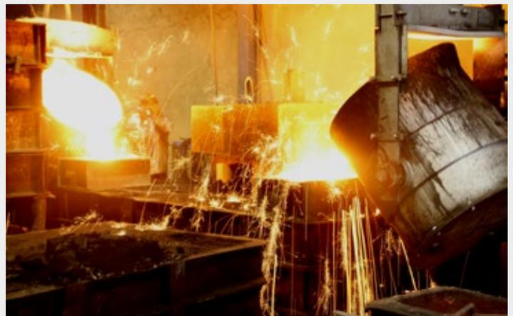
**Fig. 2:** Pouring of an 8,5 t-machine-base
