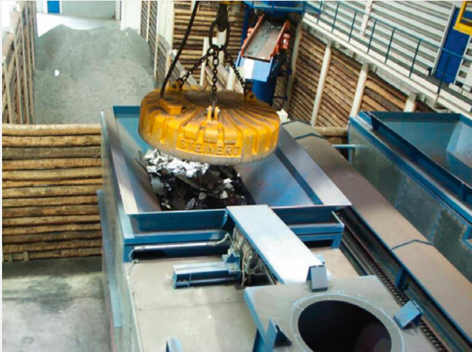
Fig. 2: Loading of a charging vehicle by magnet on crane [1]
