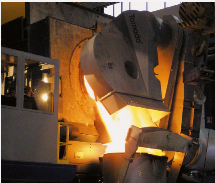
Fig. 3: Tapping a 19-t induction crucible furnace [1]
