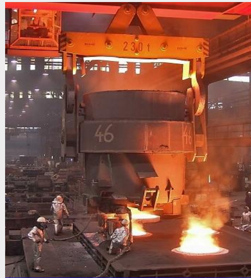
Fig. 3: Pouring from the 150 t-ladle [1]
