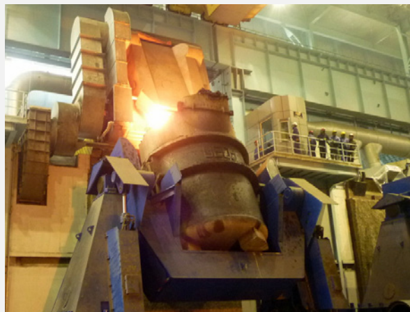
Fig. 7: Tisco-Noth: 6 x 65 t / 3 x 42 MW induction furnaces for melting ferroalloys [5]
