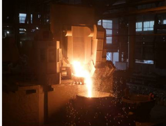
Fig. 6: Tisco-South: 2 x 30 t-/24.4 MW induction furnaces for melting ferroalloys [5]
