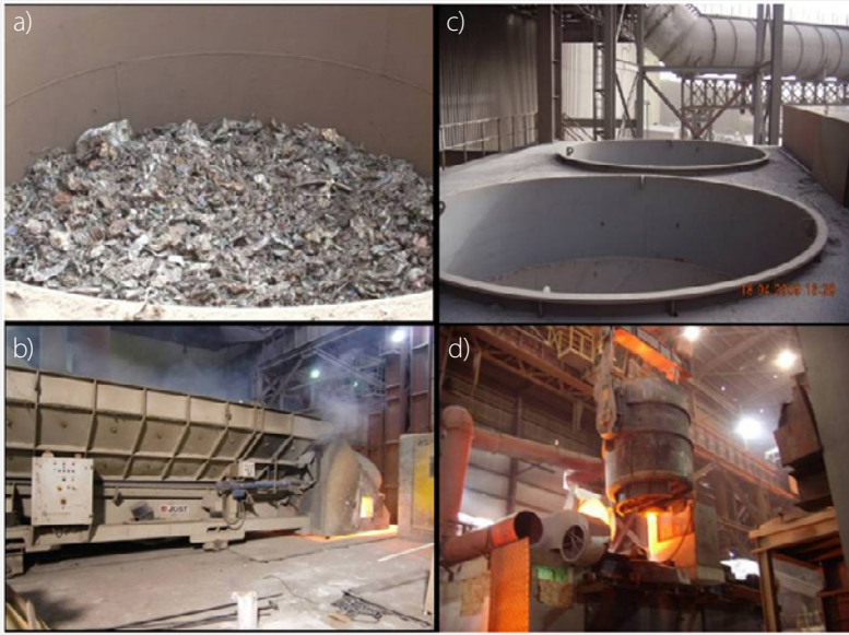
Fig. 4: 2 x 23 t-melting system at Nasco: a) Shredded scrap, b) Charging car, c) Scrap container, d) Filling of steel melt for sintering [4]
