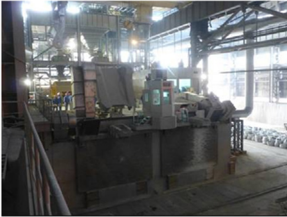
Fig. 6: Tisco-South: 2 x 30 t-/24.4 MW induction furnaces for melting ferroalloys [5]
