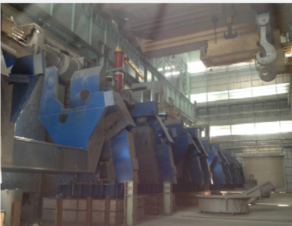
Fig. 7: Tisco-Noth: 6 x 65 t / 3 x 42 MW induction furnaces for melting ferroalloys [5]
